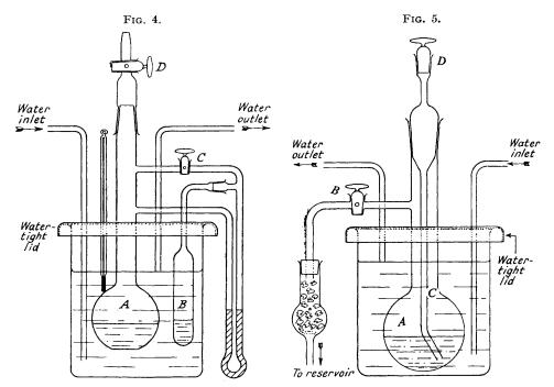
A and B respectively. The true change of pressure in A was found to approximate closely to the observed change in pressure  $\times 1.075$ , for the range of change of pressure observed.
